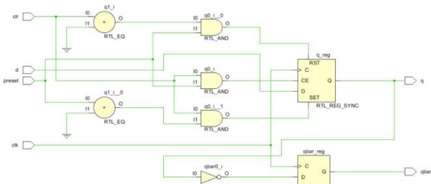
Fig. 2 Schematic Diagram of DFF
