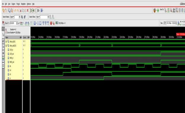
Fig. 6 Simulation waveform of 3 bit USR
