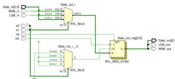
Fig. 1 Schematic Diagram of USR.
