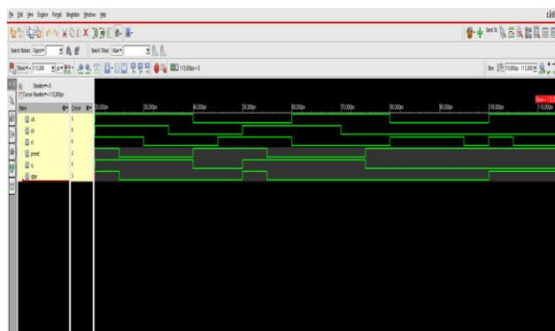
Fig. 4 Simulation waveform of DFF
