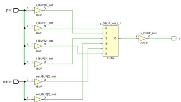
Fig. 3 Schematic Diagram of 4:1 MUX
